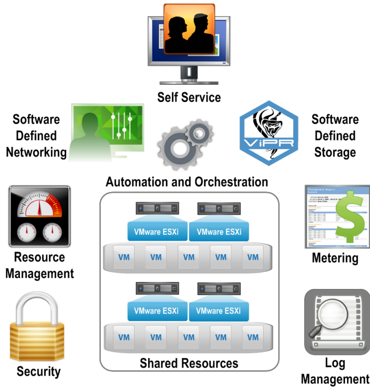
Figure 2. EMC Enterprise Hybrid Cloud features and functionality
