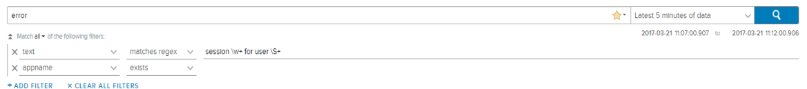
Figure 6. An example of the search bar with a keyword, a constraint with a regular expression, and a constraint with a field operation. In order for the query to return a result, all three items need to return a match.
